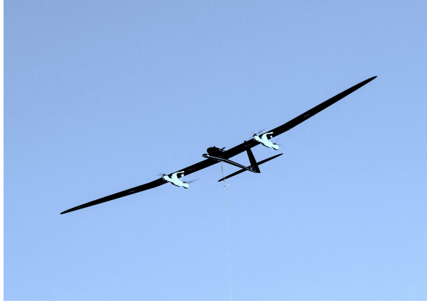
Fig. 3 5 kW prototype of Kitemill AS with vertical takeoff- and landing capabilities.
