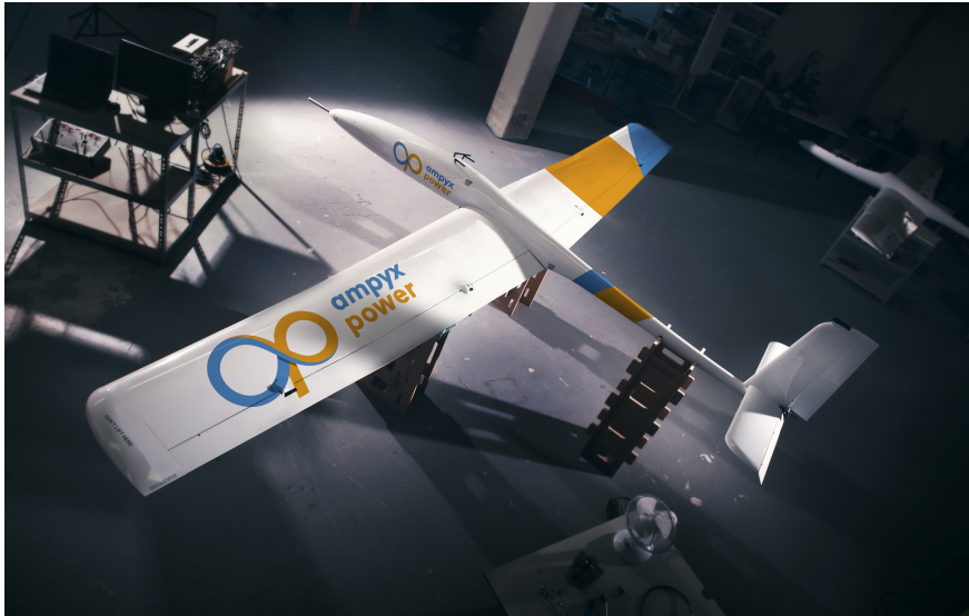
Figure 2: The 2 nd prototype high lift, rigid wing autonomous aircraft designed by Ampyx Power B.V. [5] and build in 2009.
