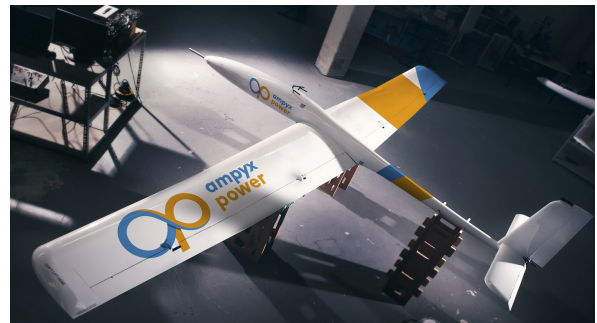
Fig. 2. The second generation PowerPlane developed by Ampyx Power B.V. with mass = 36.8 kg, wing area = 3 m 2 , wing span = 5.5 m and reference chord = 0.55 m.
