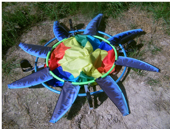
Fig. 22.20 Possible configuration of the small-scale system shown in Fig. 22.7 before vertical launch maneuver
