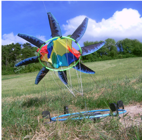
Fig. 22.7 Small-scale system built with two spars, a ring, four retractable leashes, a rotating tray, a parachute kite and semi-rigid rotor blades. The system uses four peripheral tethers and several suspension lines. The flying rotor measures 1.3 m from tip to tip
