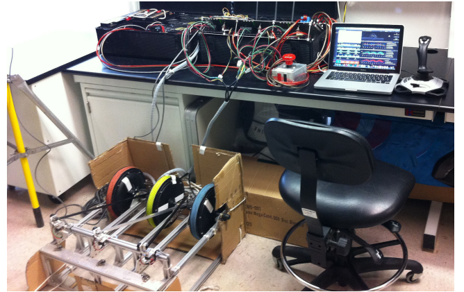
Fig. 5. VPHIL laboratory setup of the small-scale three-winches ground station prototype.
