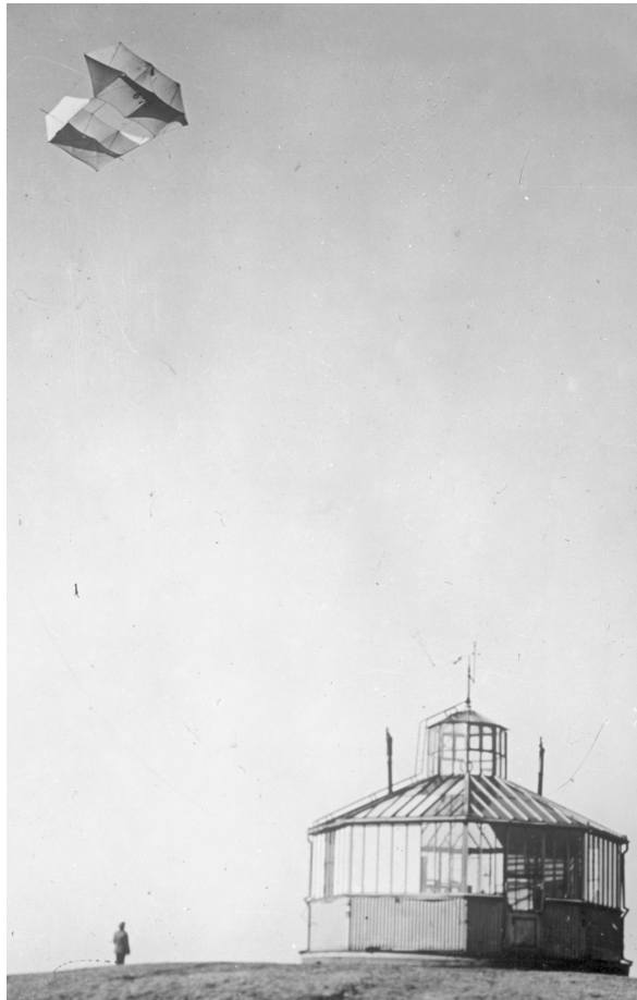
Fig. 6.1 A Lindenberg R-kite with 32 \text{ m}^2 wing surface area flying over the Lindenberg Observatory in the 1950s [22]. Designed by Rudolf Grund, this type of kite was widely used for atmospheric soundings thanks to its stable flight characteristics and its self-regulating incidence angle, which reduced wear on both the tether and the ground fixation.
