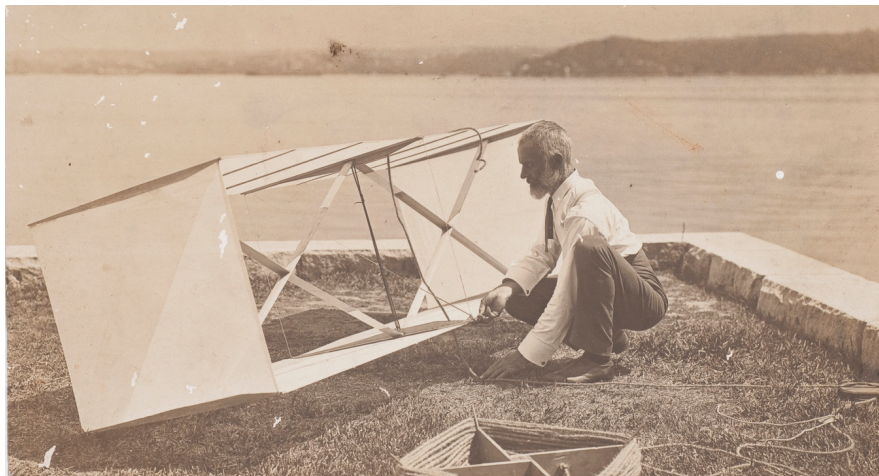
Fig. 6.5 Lawrence Hargrave working on an experimental box kite, Woollahra Point, Australia, around 1910 [27]. The box structure affords very large stability for the given structural weight. It also provides plenty of fixation surface area for instrumentation.
