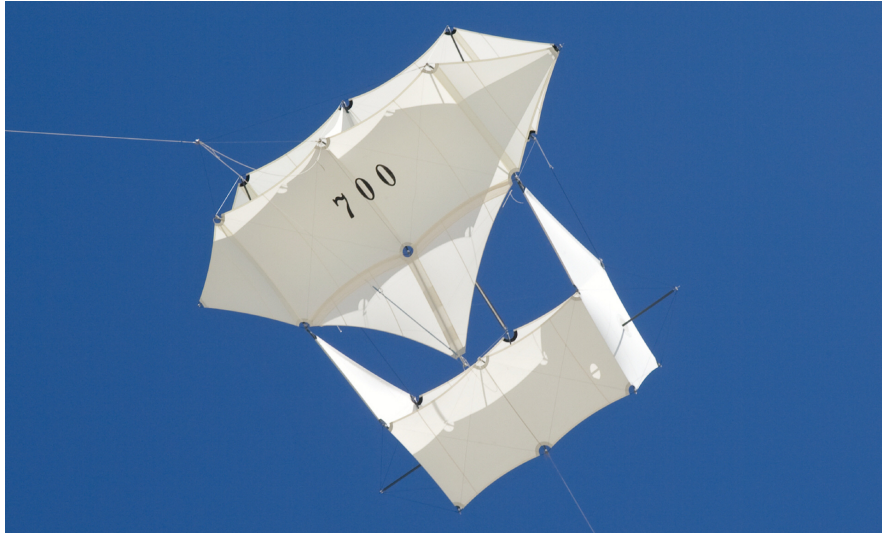
Fig. 6.10 A restored Lindenberg R-Kite with 32 \text{ m}^2 wing surface area [25]. The photo clearly displays the hinged dual-cell construction which allowed the kite to adjust to varying wind conditions.
